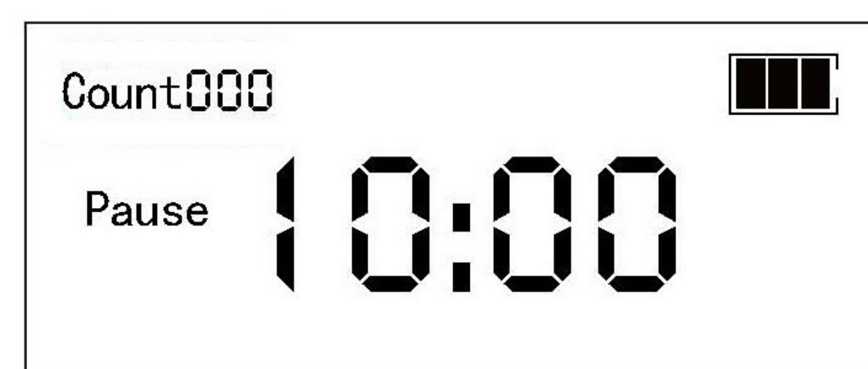
Dia. 15.2 “Pause time” display after first power connection
