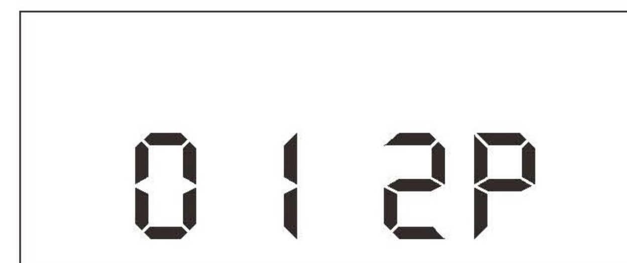
Dia. 15.5 Setting of 2P - Impulse cycles
