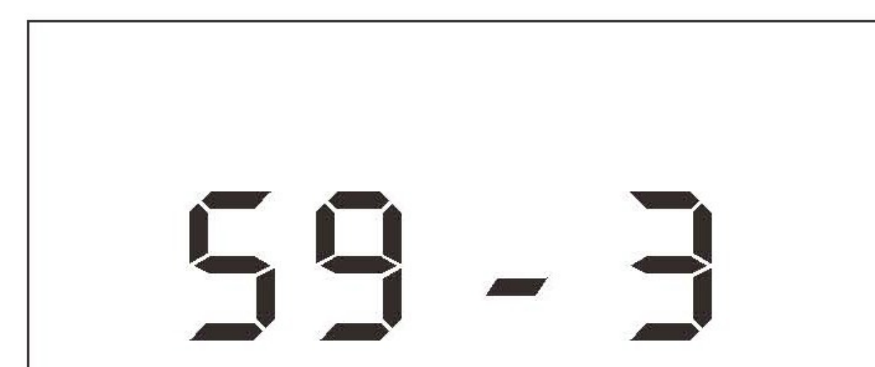
Dia. 15.7 Setting of 3P - Lube Time in Second
